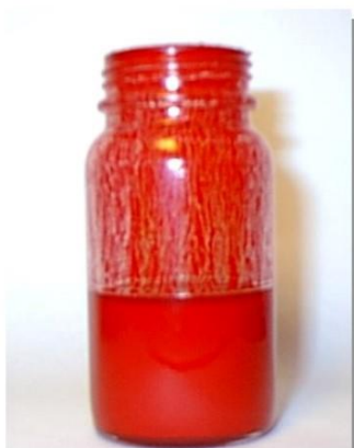
where the pigments separate and formed an un-homogenous 颜料分离并且不均匀
