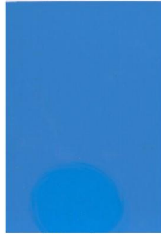
A more stabilized system. There is still some small white rub out (color turn lighter) where the white based is not sufficient stabilized. However, you can notice that the rub out area has different color tone, a high possibility that both pigments are still not sufficient stabilized.
